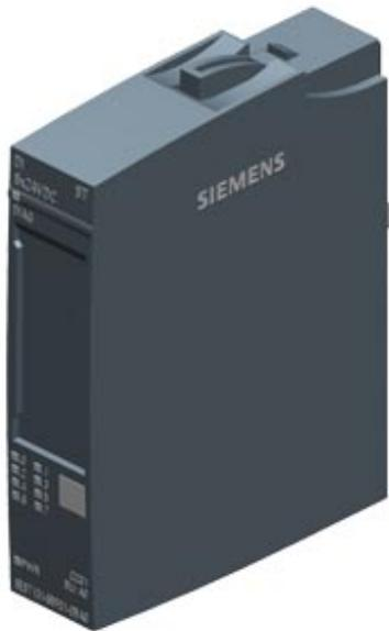
SIMATIC ET 200SP, Digital input module, DI 8x 24V DC Standard, type 3 (IEC 61131), sink input, (PNP, P-reading), Packing unit: 1 piece, fits to BU-type A0, Colour Code CC01, input delay time 0,05..20ms, module diagnostics for: short-circuit of sensor supply, wire break, supply voltage
